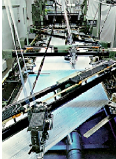
Figure 7. Multiaxis machine. Cross-plyes of +45°, 90°, -45° or angle in between 22° and 90° are laid in place by a carriage that shuttles back and forth across the width of the roll.
